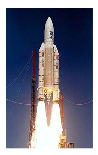
When the guidance system's own computer tried to convert one piece of data the sideways velocity of the rocket from a 64 bit format to a 16 bit format; the number was too big, and an overflow error resulted after 36.7 seconds. When the guidance system shutdown, it passed control to an identical, redundant unit, which was there to provide backup in case of just such a failure. Unfortunately, the second unit, which had failed in the identical few manner **a** milliseconds before.
