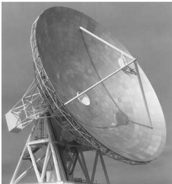
**Figure 8.7** Standard-A (C-band 6/4 GHz) 32-m antenna.
