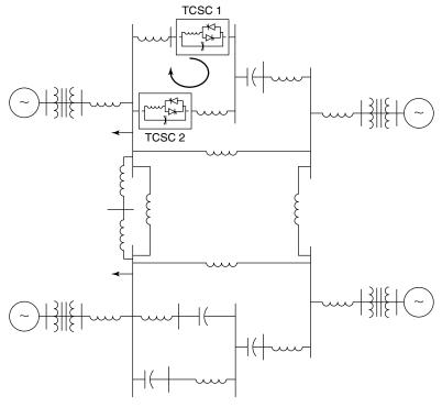
Figure 9.37 A low-loop impedance configuration with coupled TCSCs.
