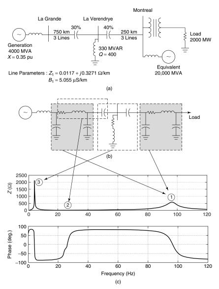
**Figure 5.42** (a) A simplified Hydro-Quebec network during degraded conditions; (b) an equivalent representation using  $\pi$  models of transmission lines; and (c) the magnitude and phase of positive-sequence impedance at the La Verendrye substation.
