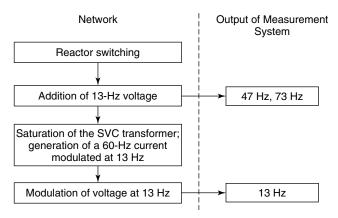
Figure 5.47 Explanation of the addition/modulation phenomenon.
