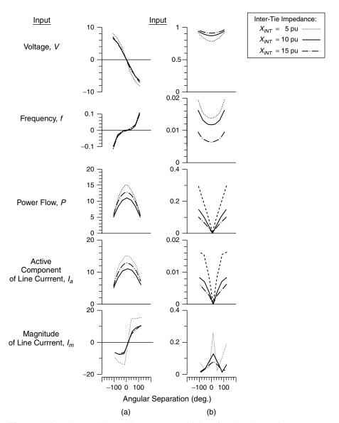
**Figure 6.14** Observability and inner-loop sensitivity of various input signals versus the inter-tie power transfer and impedance: (a) observability  $K_{OXi}$  (pu/pu) and (b) inner-loop sensitivity  $|K_{IXi}|$  (pu/pu).
