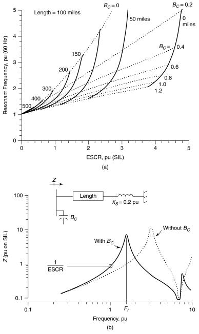
**Figure 5.14** Plots illustrating the relationships of (a) ESCR and (b)  $F_{r0}$  to parameters of a system with long lines.
