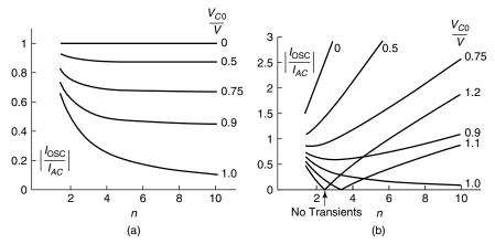
**Figure 3.29** The magnitude of the oscillatory component for different tuning of the LC branch and different precharging on C: (a) firing criterion,  $v(t) = V_{C0}$  ( $V_T = 0$ ) and (b) firing criterion, crest of vt.
