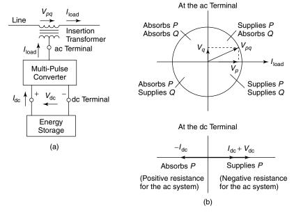
**Figure 10.18** (a) Generalized series-connected synchronous-voltage source employing a multi-pulse converter with an energy-storage device; (b) the different operating modes for real- and reactive-power exchange.
