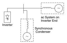
**Figure 3.2** An equivalent circuit of a synchronous condenser connected at the inverter end of a dc link.
