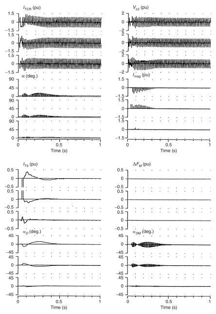
**Figure 5.39** A 3-phase fault for a weak ac system (TCR balance control with  $I_{T0}$  input only).
