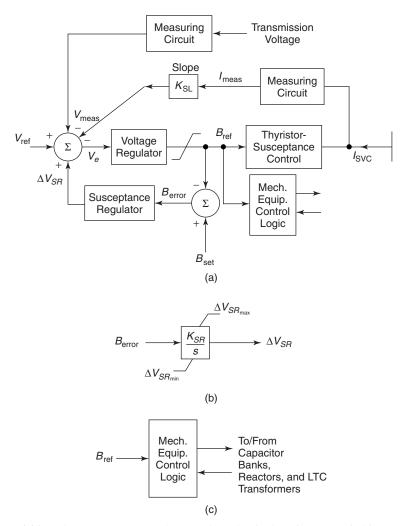
**Figure 4.22** The susceptance regulator and mechanical-equipment switching: (a) the general structure; (b) the susceptance regulator; and (c) the mechanical equipment switching.
