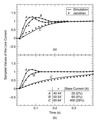
**Figure 7.20** The line-current response to equal step change in the conduction angle at different operating points for a Kayenta TCSC: (a) synchronization with capacitor voltage and (b) synchronization with line current.
