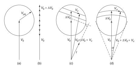
**Figure 10.26** A phasor diagram illustrating the general concept of series-voltage injection and attainable power-flow control functions: (a) series-voltage injection; (b) terminal-voltage regulation; (c) terminal-voltage and line-impedance regulation; and (d) terminal-voltage and phase-angle regulation.
