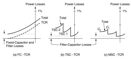
**Figure 3.42** A comparison of losses for different SVC configurations.
