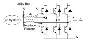
Figure 10.4 An elementary 6-pulse VSC STATCOM.
