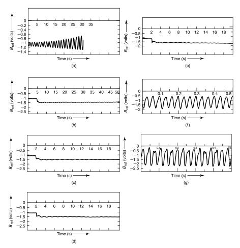
**Figure A.7** The long-duration step response of the SVC as obtained on the simulator: (a) susceptance-order  $B_{\text{ref}}$  for  $K_I = 94.4$  without the application of step input; (b)  $K_I = 198.7$ ; (c)  $K_I = 632$ ; (d)  $K_I = 1415$ ; (e)  $K_I = 2831$ ; (f) susceptance-order  $B_{\text{ref}}$  for  $K_I = 4246$  without the application of step input; and (g) susceptance-order  $B_{\text{ref}}$  for  $K_I = 6321$  without the application of step input.
