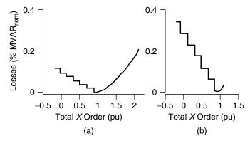
**Figure 7.18** The losses in a multimodule TCSC: (a)  $I_{\text{line}} = 1/2I_{\text{rated}}$  and (b)  $I_{\text{line}} = I_{\text{rated}}$ .
