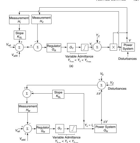
**Figure 5.8** (a) A block diagram of the system voltage controller incorporating an SVC and (b) a simplified block diagram of the system voltage controller for  $V \simeq V_{\text{rated}}$ .
