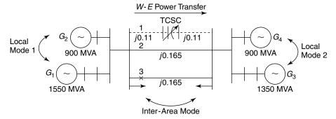
Figure 8.10 A two-area, four-machine system.
