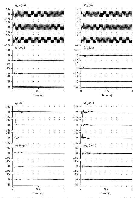
**Figure 5.41** A 3-phase fault for a weak ac system (TCR balance control with both  $I_{T0}$  and  $\Delta F_M$  inputs).
