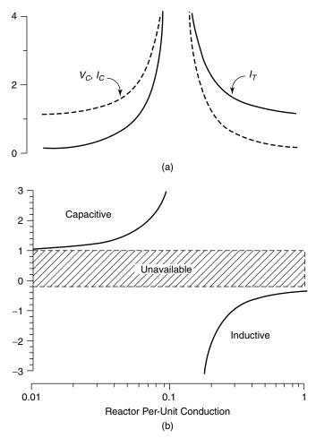
**Figure 7.7** Variation of the TCSC voltage, currents, and reactance with per-unit TCR conduction: (a) currents (pu on  $I_{\text{line}}$ ), voltage (pu on  $X_C \cdot I_{\text{line}}$ ); (b)  $X_{\text{net}}$  (pu on  $X_C$ ).
