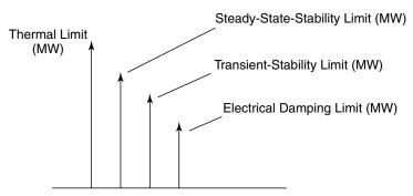
**Figure 6.7** Comparison of different limits on the power flow.
