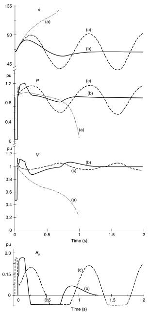
**Figure 6.6** The system response for severe disturbance,  $P_0 = 0.9$  pu: curve (a) without SVC; curve (b) with SVC (0.27-pu capacitance/0.07-pu inductance) with the optimum control strategy; and curve (c) with SVC (0.27-pu capacitance/0.07-pu induction) with the constant-voltage control strategy.
