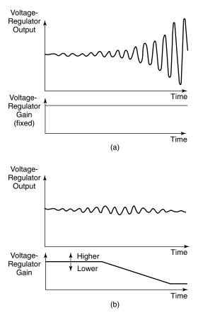
**Figure 5.26** Behavior of the SVC voltage controller: (a) without gain-supervisor control and (b) with gain-supervisor control.
