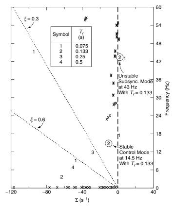
**Figure 9.13** The effect of the SVC response rate on system eigenvalues for a mostly series-compensated system due to a 2-line loss south of La Verendrye.
