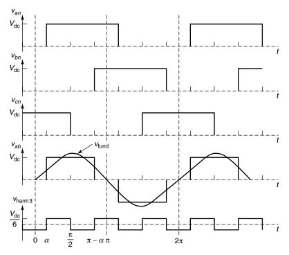
**Figure 10.5** An ac line-voltage output of a 6-pulse voltage-source inverter for a 180° conduction sequence.
