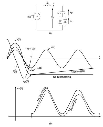
Figure 3.31 Voltages after turn-off to the TSC: (a) a circuit diagram and (b) the voltage-current waveforms.
