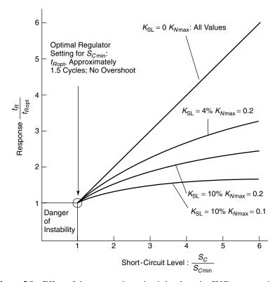
**Figure 5.9** Effect of the system short-circuit level on the SVC response time.
