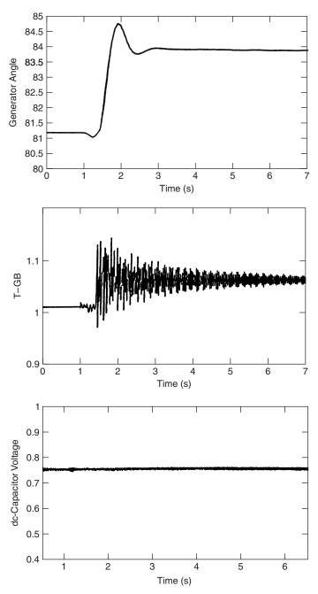
**Figure 10.24** The SSSC response for a step change in the mechanical input of an HP turbine.
