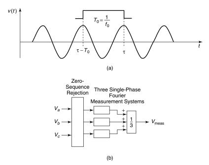
**Figure 4.4** (a) The principle of operation of a single-phase Fourier measurement system and (b) a 3-phase Fourier measurement system.
