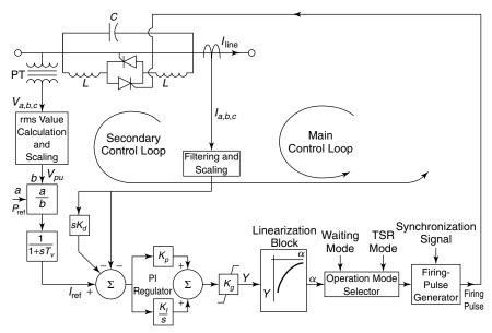
Figure 8.8 An enhanced TCSC power-control structure.
