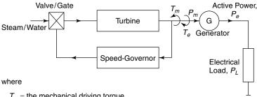
$T_m$  = the mechanical driving torque
