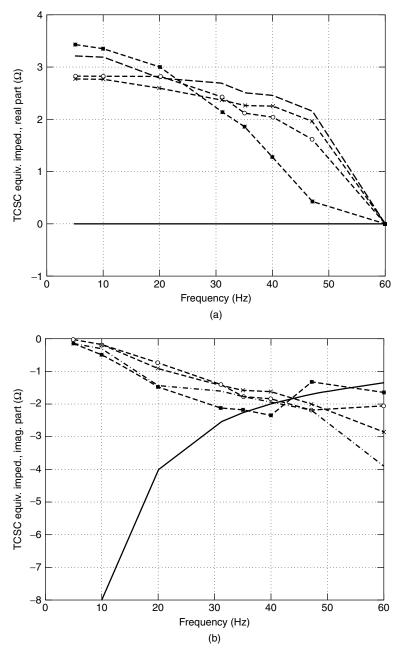
**Figure 8.22** Frequency-domain characteristics of (a) the real part and (b) the imaginary part of the TCSC equivalent impedance, where —— is the TCSC internal capacitor and the  $X_{\text{order}}$  is as follows: ----=1.5; ----=1.5; ----=2.1; and ----=2.9.
