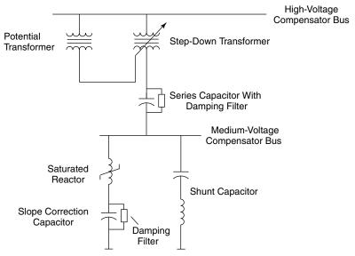
Figure 3.4 An SR compensator.
