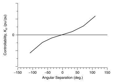
**Figure 6.12** Controllability  $K_{ci}$  as a function of inter-tie power transfer.
