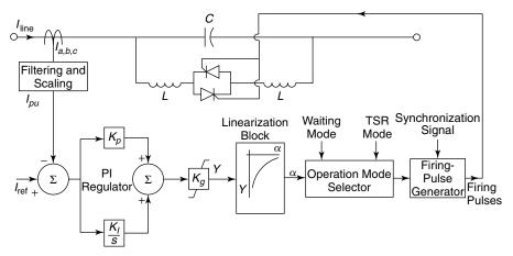
**Figure 8.2** A TCSC constant-current (CC) controller model.
