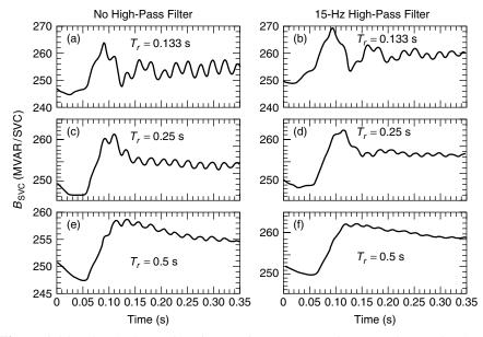
**Figure 9.16** The SVC transient in a series-compensated system due to the SVC response rate and the high-pass filter (the regulator output is at Chibougamau).
