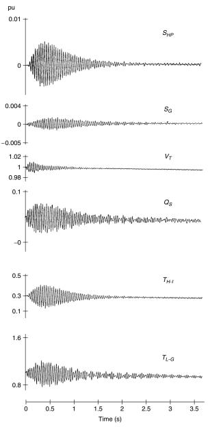
**Figure 6.23** Damping of torsional mode 3 with an SVC, where  $S_{\rm HP}$  = the speed deviation of the HP turbine rotor mass;  $S_G$  = the speed deviation of the generator rotor mass;  $V_T$  = the generator terminal voltage;  $Q_s$  = the SVC reactive power;  $T_{H-I}$  = the mechanical shaft torque in HP-IP section; and  $T_{L-G}$  = the mechanical shaft torque in LP-GEN section.
