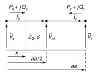
**Figure 2.4** The power on a lossless distributed line.
