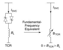
**Figure 3.15** A simple SVC circuit using a TCR.
