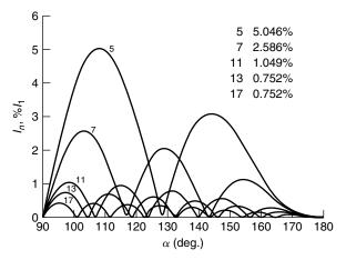
Figure 3.9 Harmonics in a TCR current.
