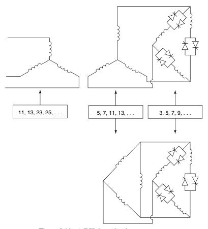
**Figure 3.14** A TCR in a 12-pulse arrangement.
