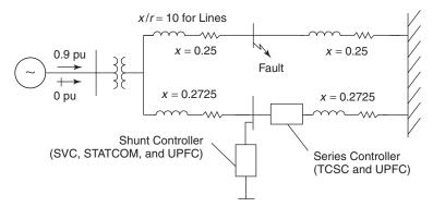
Figure 10.31 A study system for transient-stability evaluation.
