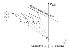
**Figure 3.34** The operating characteristic of a TSC.
