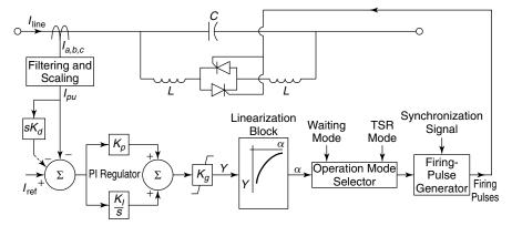
**Figure 8.6** An optimized TCSC CC structure.
