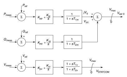
**Figure 10.35** The UPFC control system with both series real- and reactive-power flow control and shunt control for bus-voltage regulation:  $K_{pp} = 0.05$ ,  $K_{ip} = 5.0$ ,  $T_{1m} = 0.01$ ,  $T_{2m} = 0.01$ ,  $K_{pq} = 0.05$ ,  $K_{iq} = 1.2$ ,  $K_{pv} = 0.05$ ,  $K_{iv} = 0.5$ ,  $T_{1v} = 0$ , and  $T_{2v} = 0$ .
