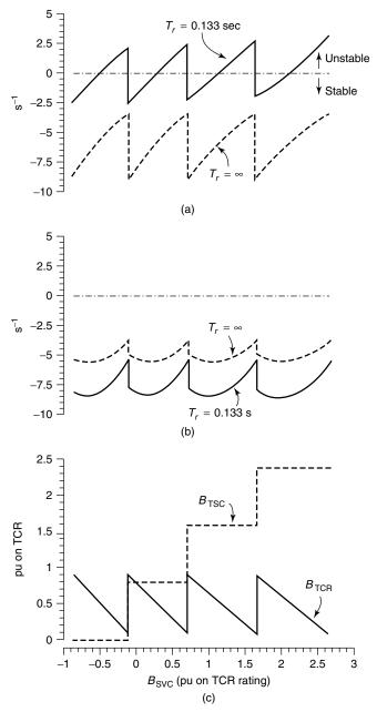
**Figure 5.52** Damping of the shunt-reactor modes versus the SVC operating point (30% series compensation, 15-Hz shunt-reactor mode): (a)  $\sigma$  of the positive-sequence mode (45 Hz); (b)  $\sigma$  of the negative-sequence mode (75 Hz); and (c) the SVC operating point.
