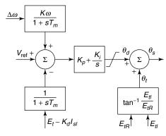
Figure 10.10 A STATCOM controller for damping the SSR.
