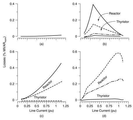
**Figure 7.17** The losses in a single-module TCSC: (a) blocked or  $X_{\text{net}} = 1$  pu; (b) the maximum capacitive vernier; (c) the bypassed; and (d) the maximum inductive vernier.
