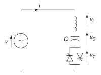
Figure 3.27 A TSC with a series reactor.
