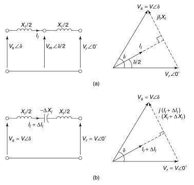
Figure 2.13 The series compensation of a short, symmetrical transmission line.
