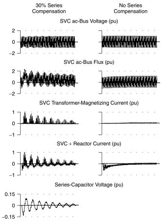
Figure 5.46 Reactor switching with and without series compensation.
