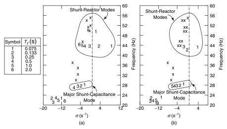
**Figure 9.15** Effect of the high-pass filter on subsynchronous modes for a mostly series-compensated La Verendrye system (contingency at 280 MVAR/SVC): (a) with no high-pass filter and (b) with a 15-Hz high-pass filter.
