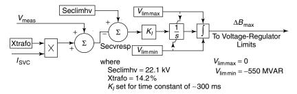
**Figure 4.25** The secondary-overvoltage limiter.
