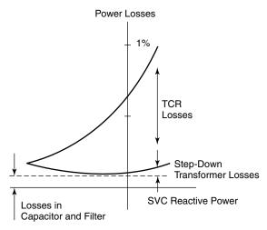
**Figure 3.24** Losses in an FC–TCR. (*Courtesy:* The CIGRE.)
