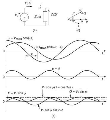
**Figure 2.1** The electrical parameters in an ac network.
