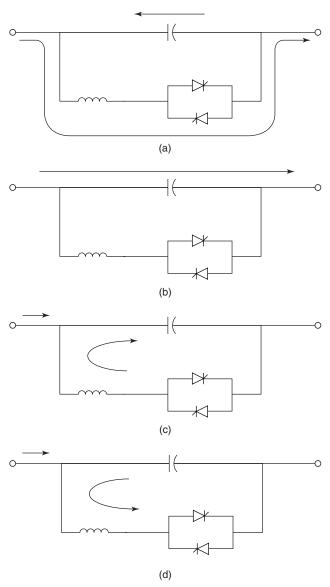
**Figure 7.4** Different operating modes of a TCSC: (a) the bypassed-thyristor mode; (b) the blocked-thyristor mode; (c) the partially conducting thyristor (capacitive-vernier) mode; and (d) the partially conducting thyristor (inductive-vernier) mode.
