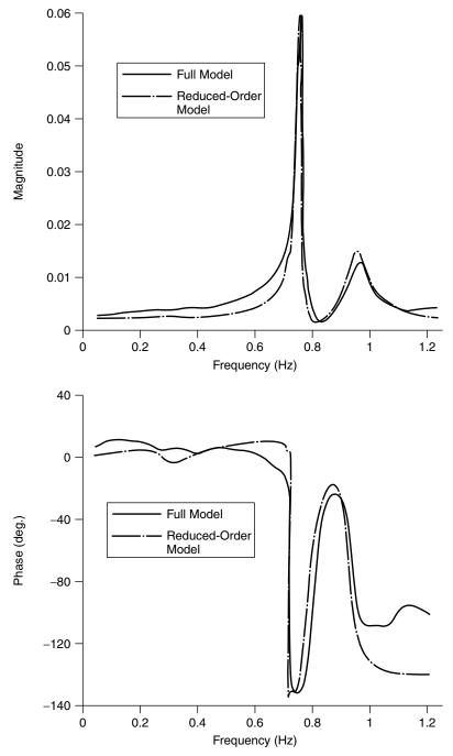
Figure 8.16 The frequency response of Edie voltage/TCSC input.
