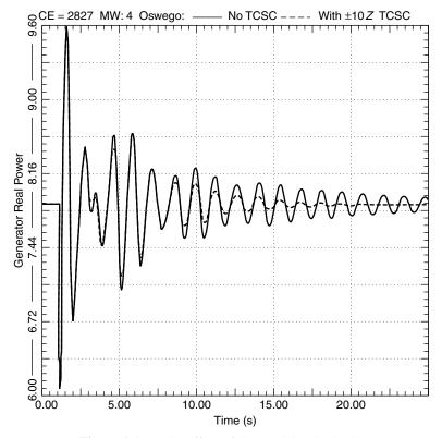
**Figure 8.17** The effect of the modulated TCSC.
