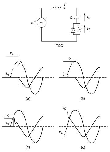
**Figure 3.30** The switching strategy for a TSC: (a) firing at the minimum valve voltage,  $v_C > v$ ; (b) firing at the zero valve voltage,  $v_C = v$ ; (c) firing at the zero valve voltage,  $v_C < v$ ; and (d) firing at the zero valve voltage,  $v_C = 0$ .
