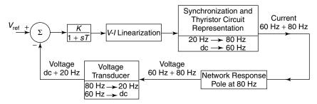
**Figure 5.11** An 80-Hz instability in the SVC control loop.
