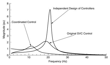
**Figure 9.24** The frequency response of SVC 1.
