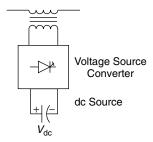
**Figure 1.9** A 1-line diagram of a static synchronous series compensator (SSSC).
