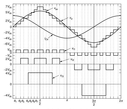
Figure 10.12 Typical voltages of the 3-level BVSI.
