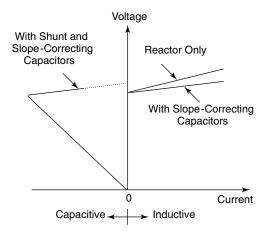
Figure 3.5 The operating characteristics of an SR compensator.
