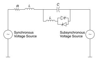
**Figure 8.18** Network for the simulation study of the TCSC equivalent impedance.
