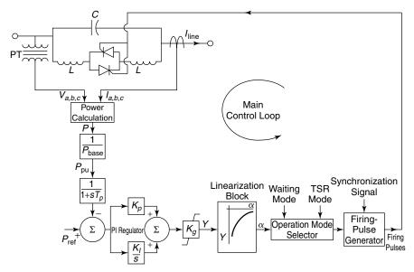
**Figure 8.7** A conventional TCSC power-control structure.
