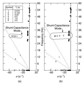
**Figure 9.25** The effect of the Radisson–Nicolet HVDC on SVC interaction for a mostly series wintertime network (280 MVAR/SVC): (a) with no HVDC and (b) with HVDC.
