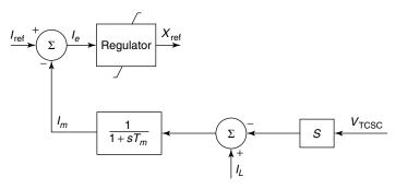
Figure 8.4 A block diagram of a CC or CA controller.
