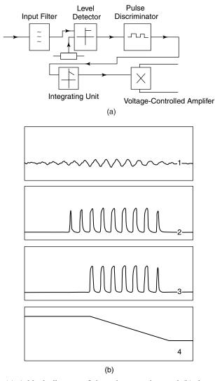
**Figure 5.25** (a) A block diagram of the gain supervisor and (b) the gain-supervisor signals: (1) input signal; (2) output from the pulse detector; (3) output from the pulse discriminator (two pulses deleted); and (4) the signal proportional to the gain reduction.
