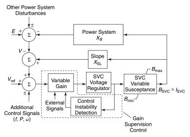
**Figure 5.24** The connection of gain-supervisor control to the SVC voltage-control system  $(V \simeq V_{\text{rated}})$ .
