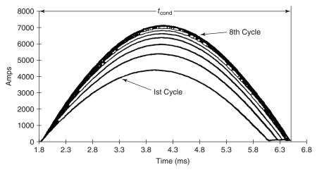
Figure 7.19 Cycle-by-cycle buildup of TCR inductor current.
