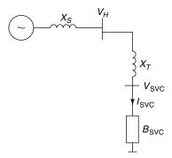
**Figure 5.5** Representation of the power system and the SVC, including the coupling transformer.
