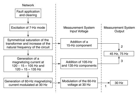
**Figure 5.50** A schematic explanation of the addition and transformer-saturation phenomena at fault application and clearing.
