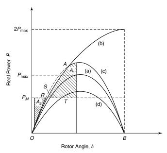
**Figure 6.5** Power-angle curves of a SMIB system: curve (a) for an uncompensated case; curve (b) with an ideal midpoint-connected SVC; curve (c) with a midpoint-connected fixed capacitor; and curve (d) with a midpoint-connected fixed inductor.
