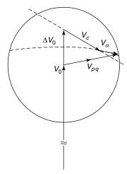
**Figure 10.27** A phasor diagram illustrating the simultaneous regulation of the terminal voltage, line impedance, and phase angle by appropriate series-voltage injection.
