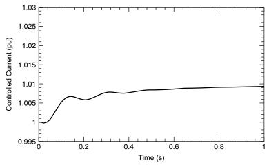
**Figure 9.43** The response of TCSC 1 to the reference-current step input with coordinated control of both TCSCs.
