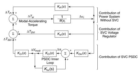
**Figure 6.10** A simplified block diagram showing the damping- and synchronizing-torque contributions of the different controllers on the *i*th power-swing mode.
