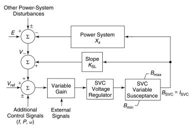
**Figure 5.21** The SVC voltage controller with variable gain  $(V \simeq V_{\text{rated}})$ .
