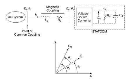
Figure 10.7 A typical STATCOM connection to the ac system.
