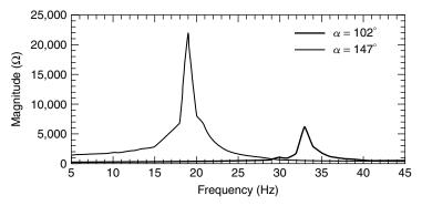
**Figure 9.2** The impedance magnitude of the SVC frequency response.
