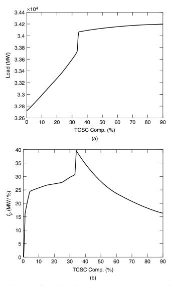
**Figure 8.29** The effect of changing the TCSC compensation levels for the critical line: (a) the loading margin and (b) the performance measure,  $f_p$ .
