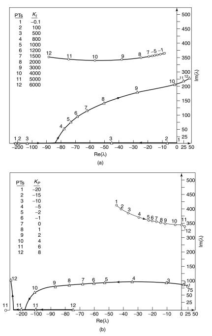
**Figure A.2** (a) The root loci of a simplified model with varying  $K_I$  ( $K_P = 0$ ) and (b) the root loci of a simplified model with varying  $K_P$  ( $K_I = 1200$ ).
