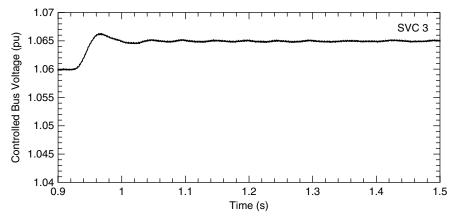
Figure 9.34 An independently optimized SVC controller.
