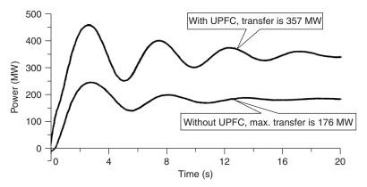
Figure 10.29 Power-transfer capability with the UPFC.
