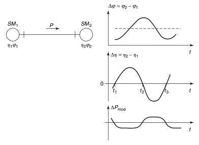
**Figure 8.9** The TCSC line-power modulation for damping enhancement.
