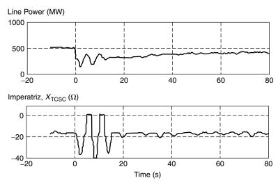
**Figure 8.38** Tripping of 300-MW generation in Tucurui, with the phasor POD in Imperatriz and the Serra da Mesa enabled.
