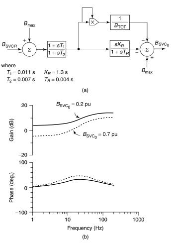
**Figure 5.29** (a) A block diagram and (b) transfer function  $(\Delta B_{\text{SVC}_0}/\Delta B_{\text{SVC}_R})$  of a nonlinear series-dynamic compensator for the SVC voltage regulator.
