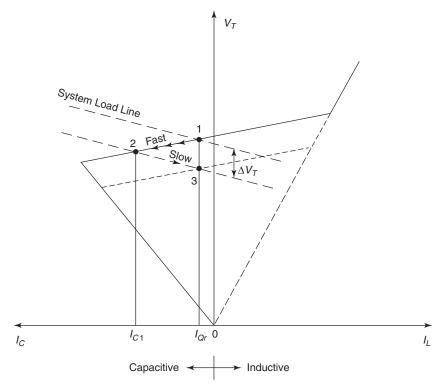
Figure 4.23 Operation of the SVC susceptance regulator.
