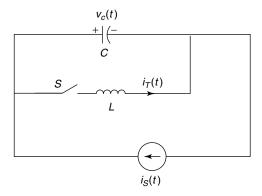
**Figure 7.5** A simplified TCSC circuit.
