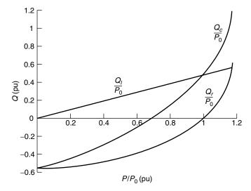
Figure 2.6 The reactive-power flows at the receiving end.
