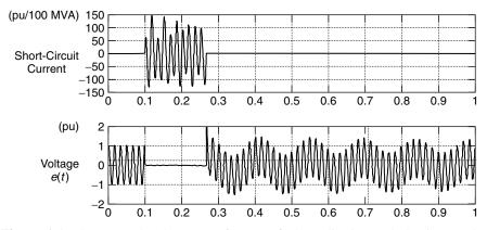
**Figure 4.6** Current and voltage waveforms at fault application and clearing on the circuit.
