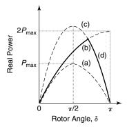
**Figure 6.3** Power-angle curves of a SMIB system: curve (a) for an uncompensated case; curve (b) for an ideal midpoint SVC with unlimited rating ( $Q_{SVC} > 4P_{max}$ ); curve (c) for a fixed capacitor connected at its midpoint; and curve (d) for a midpoint SVC with limited rating ( $Q_{SVC} \approx 2P_{max}$ ).
