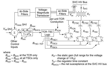
**Figure 5.6** Basic elements of SVC voltage-regulation control with TSC.
