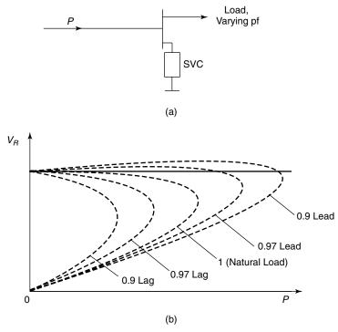
**Figure 6.24** (a) An SVC connected at the load bus by a radial transmission line supplying a load and (b) the voltage profile at the receiving end of a loaded line with a varying power factor load.
