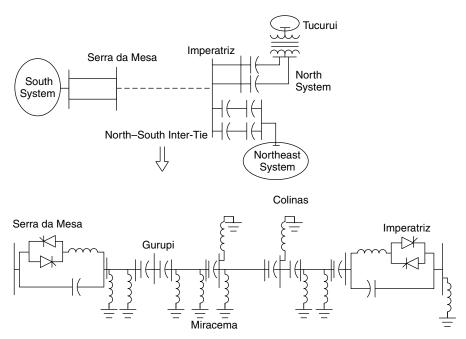
Figure 8.31 Single-line diagram of the Imperatriz–Serra da Mesa transmission line.
