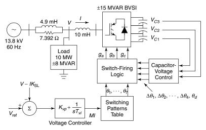
**Figure 10.15** Distribution-system compensation using a BVSI STATCOM.
