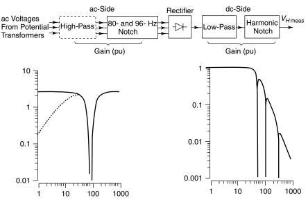
**Figure 4.10** The filtering of measurement voltages (solid lines represent existing filters; dashed lines represent additional filters needed for series-compensated ac lines).
