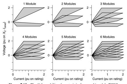
**Figure 7.13** The *V-I* capability characteristic for a multimodule TCSC.
