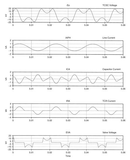
**Figure 7.8(b)** TCSC waveforms in the inductive mode of operation ( $\alpha = 130^{\circ}$ ).
