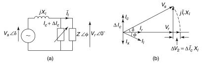
Figure 2.3 The reactive-power control for voltage regulations.
