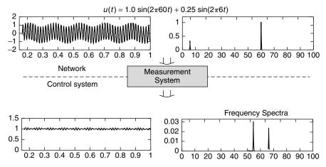
**Figure 4.8** The measurement technique and frequency spectrum obtained by using Fourier analysis.
