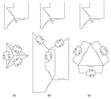
**Figure 3.18** Various arrangements of a TCT compensator: (a) star-connected reactors and a delta-connected thyristor controller; (b) star-connected reactors in series with a thyristor controller; and (c) delta-connected reactors and a thyristor controller.
