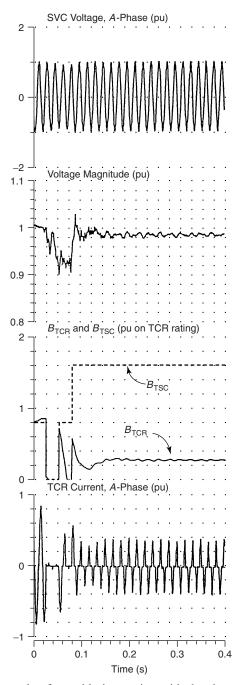
**Figure 5.56** An example of unstable interaction with the shunt-reactor mode with a 15-Hz high-pass filter.
