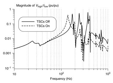
**Figure 9.27** Driving-point impedance at the Fraser bus for a base-case-system model with and without TSCs.
