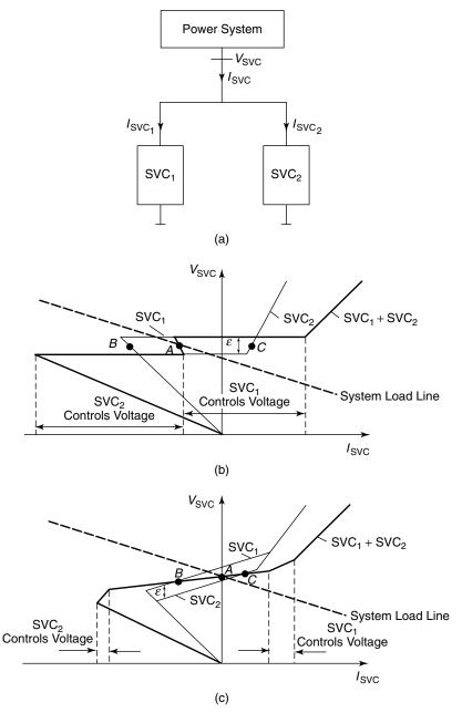
**Figure 5.4** (a) Two parallel-connected SVCs at a system bus; (b) two SVCs in parallel with difference  $\epsilon$  in the reference-voltage setpoints without current droop; and (c) two SVCs in parallel with current droop and with difference  $\epsilon$  in the reference-voltage setpoints.
