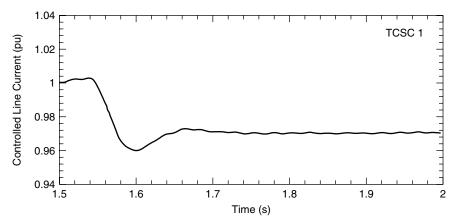
Figure 9.33 An independently optimized TCSC controller.
