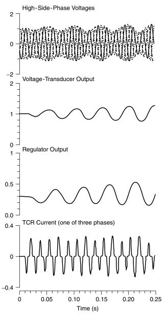
Figure 5.12 An example of SVC voltage-regulator instability.
