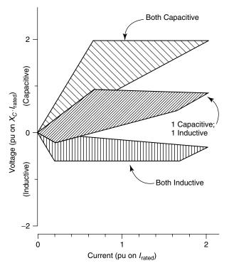
Figure 7.12 The V-I capability characteristics for a two-module TCSC.
