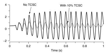
Figure 8.27 Benefit of the TCSC to damp transient-shaft torques.
