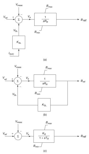
**Figure 4.15** Alternative implementations of current droop (slope) in the voltage regulator: (a) an integrator with current-droop feedback; (b) an integrator with susceptance-droop feedback; and (c) a gain–time constant.
