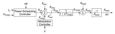
**Figure 7.22** A block diagram of the variable-reactance model of the TCSC.
