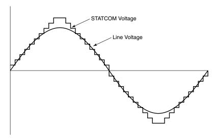
**Figure 10.6** The output voltage of a 48-pulse STATCOM that generates reactive power.
