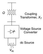
**Figure 1.8** A GTO-based static synchronous compensator (STATCOM).
