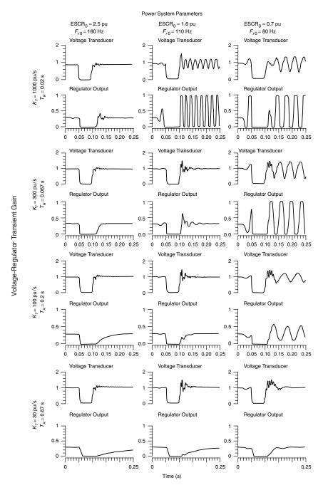
**Figure 5.15** Effect of power-system characteristics on SVC transient response with  $B_{T0} = 0.3$  pu.
