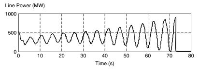
**Figure 8.35** Tripping of 300-MW generator in Tucurui, with the lead-lag and phasor PODs both disabled.
