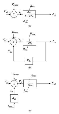
**Figure 5.7** Alternate voltage-regulator forms: (a) a gain–time constant; (b) an integrator with susceptance-droop feedback; and (c) an integrator with current-droop feedback.
