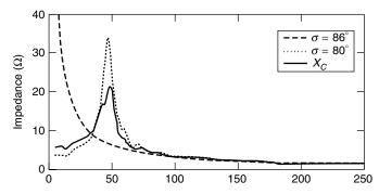
**Figure 9.5** The impedance-magnitude plot of the TCSC frequency response.
