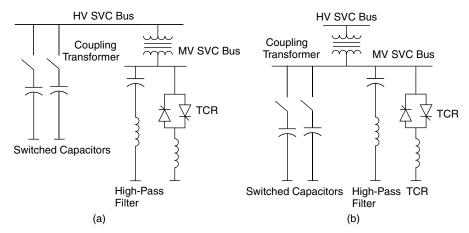
**Figure 3.25** Different configurations of an MSC–TCR compensator.
