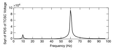
**Figure 8.20** The square root (sqrt) of the power-density spectrum (PDS) of the simulated TCSC voltage.
