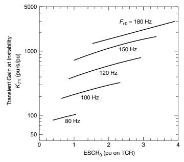
**Figure 5.20** Transient gain at instability versus the power-system parameters with  $B_{T0} = 0.3$  pu.
