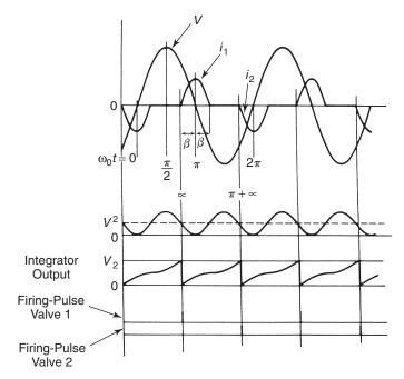
Figure 4.19 Waveforms for a single-phase TCR.
