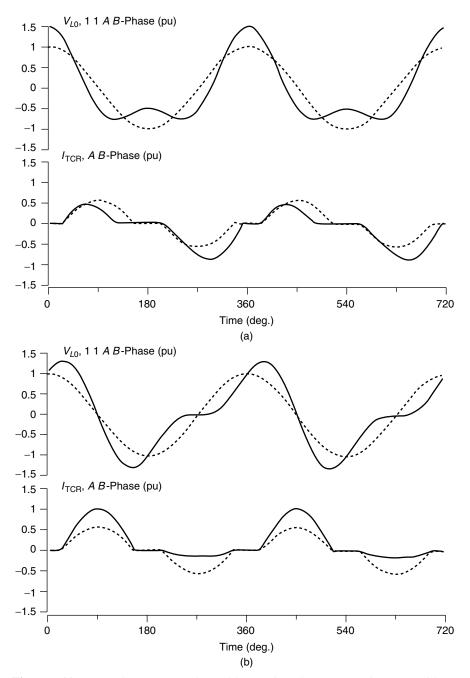
**Figure 5.32** Natural response to the 2nd harmonic voltage: (a)  $V_2$  in phase with  $V_1$  and (b)  $V_2$  lagging behind  $V_1$  by  $90^{\circ}$ .
