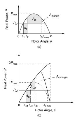
**Figure 6.4** Power-angle curves depicting transient-stability margins in the SMIB system: (a) the uncompensated system and (b) the SVC-compensated system.
