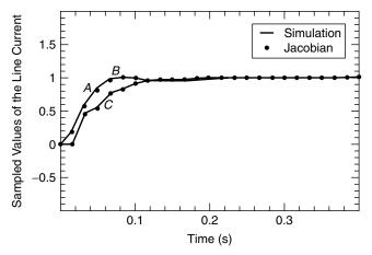
**Figure 7.26** Response of the closed-loop, conduction-angle controller.
