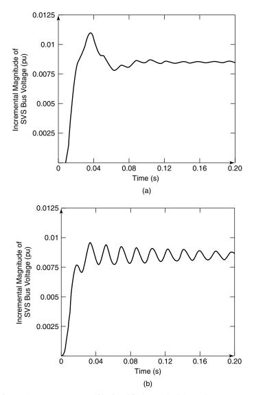
**Figure A.5** The step responses of a simplified model with varying  $K_P$ : (a)  $K_P = -3$  and (b)  $K_P = 3$ .
