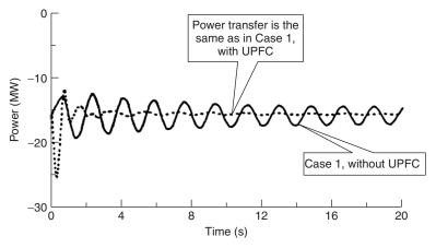
**Figure 10.30** A comparison of oscillation damping.
