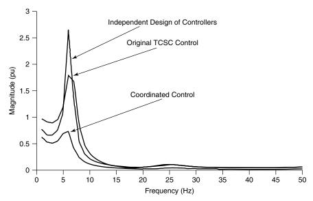
Figure 9.44 The frequency response of TCSC 1.
