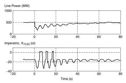
**Figure 8.37** Tripping of 300-MW generator in Tucurui, with the phasor POD in Imperatriz and the Serra da Mesa disabled.
