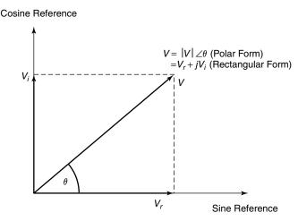
**Figure 4.14** The phasor determination via projections.
