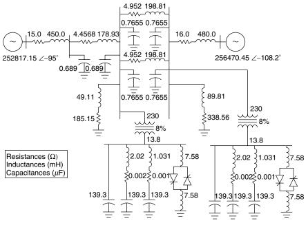
**Figure 9.17** A study system for the analysis of high-frequency interaction between SVCs.
