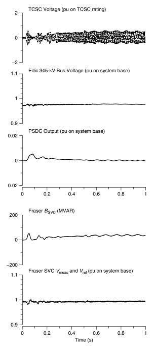
**Figure 9.30** The TCSC and SVC response to TCSC insertion with a modified voltage-input PSDC.
