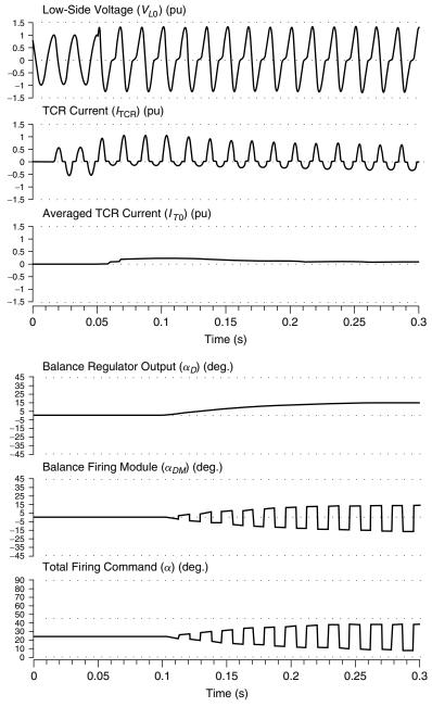
**Figure 5.38** Natural response to the 2nd harmonic voltage for 50%  $V_2$  that is 90° out of phase with  $V_1$  (TCRBC is released at 0.1 s).
