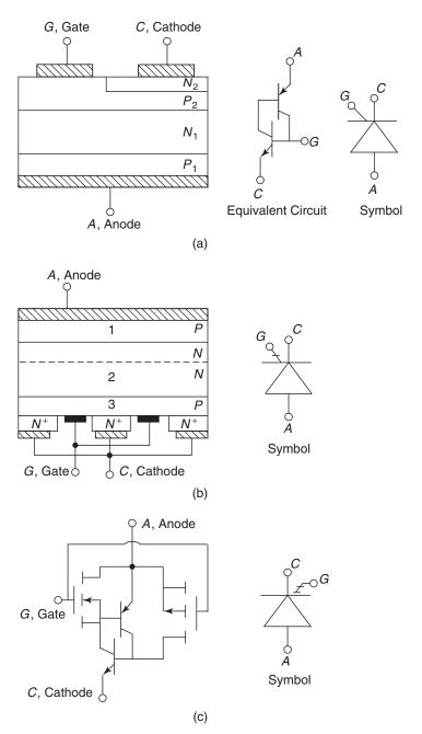
**Figure 1.5** Semiconductor switching devices for power-electronics applications: (a) a thyristor (silicon-controlled rectifier); (b) a gate turn-off (GTO) thyristor; and (c) a P-MCT equivalent circuit.
