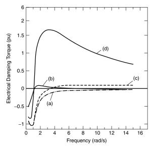
**Figure 6.21** The electrical damping torque for an SVC voltage controller and different auxiliary controllers: (a) the voltage controller; (b) the line-reactive power; (c) the bus frequency; and (d) the CIF.
