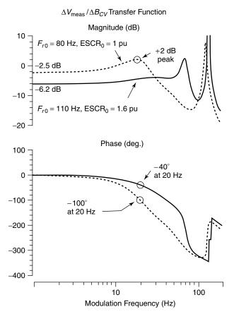
**Figure 5.16** Effect of power-system response characteristics on voltage-sensitivity transfer function.
