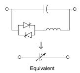
**Figure 1.7** A thyristor-controlled series capacitor (TCSC).
