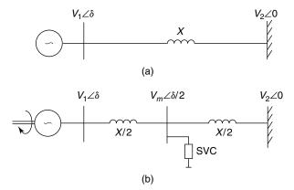
**Figure 6.1** The single-machine infinite-bus (SMIB) system: (a) an uncompensated system and (b) an SVC-compensated system.
