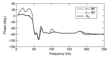
**Figure 9.6** The impedance-angle plot of the TCSC frequency response.
