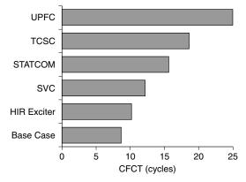
**Figure 10.36** Comparative evaluation of the CFCT.
