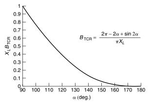
**Figure 3.8** Control characteristics of the TCR susceptance,  $B_{TCR}$ .
