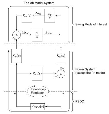
**Figure C.1** Multimodal-decomposition block diagram.
