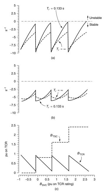
**Figure 5.55** Damping of the shunt-reactor modes versus the SVC operating point with a 15-Hz high-pass filter (30% series compensation, 15-Hz shunt-reactor mode).
