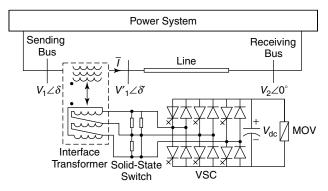
**Figure 10.20** A line compensated with an SSSC.
