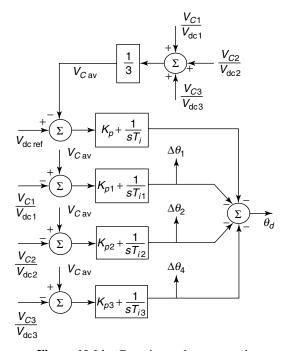
Figure 10.14 Capacitor-voltage control.
