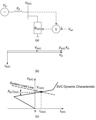
**Figure 5.2** (a) A simplified block diagram of the power system and SVC control system; (b) a phasor diagram of the ac system for the inductive SVC current; and (c) characteristics of the simplified power system and the SVC.
