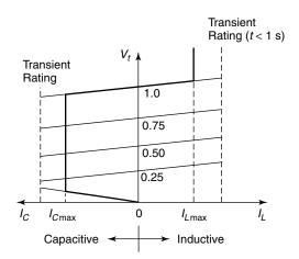
**Figure 10.2** The *V-I* characteristic of the STATCOM.
