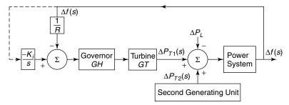
**Figure 1.2** An AGC with supplementary control on the principal generating unit.
