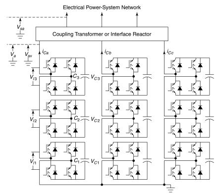
Figure 10.11 The 3-phase, star-connected 3-level BVSI.
