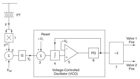
**Figure 4.18** Phase-locked oscillator control for a single-phase TCR with (voltage)<sup>2</sup> feedback.
