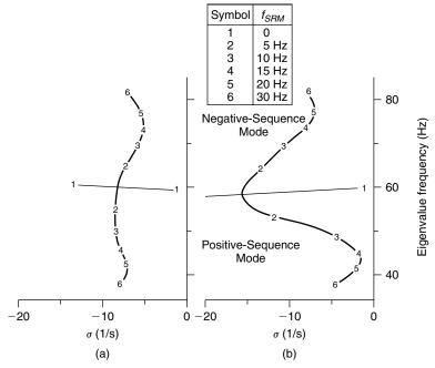
**Figure 5.51** Root locus with varying shunt-reactor size for 30% series compensation (the SVC is at zero net output with one TSC and a near-full-conduction TCR): (a) no-SVC voltage regulator and (b) fast-SVC voltage regulator.
