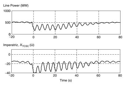
**Figure 8.36** Tripping of 300-MW generator in Tucurui, with the lead-lag POD in Impertriz and the Serra da Mesa disabled.
