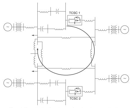
**Figure 9.38** A high-loop impedance configuration with uncoupled TCSCs.
