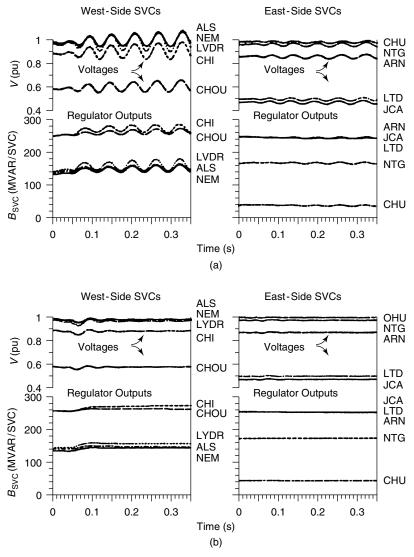
**Figure 9.9** The SVC transient behavior in La Verendrye system due to "snapshot" reactor switching at Abitibi. (a) The existing SVC response rate ( $T_r = 0.133$  s) and (b) the reduced SVC response rate ( $T_r = 0.5$  s).
