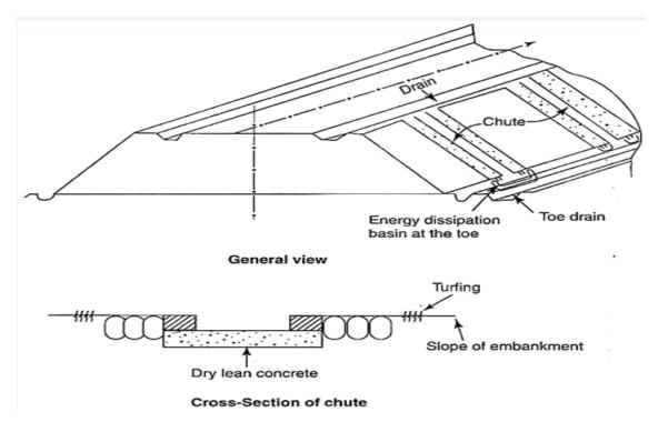
Fig. Drainage system for high Embankment
