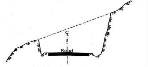
Typical Cross Sections of Box cutting
