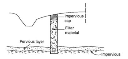
Fig. Subsurface drain to intercept drain water
