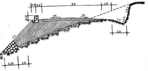
Typical Cross Sections of Cut and fill
