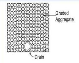
Fig. Geosynthetic-encased aggregate drain with a pipe
