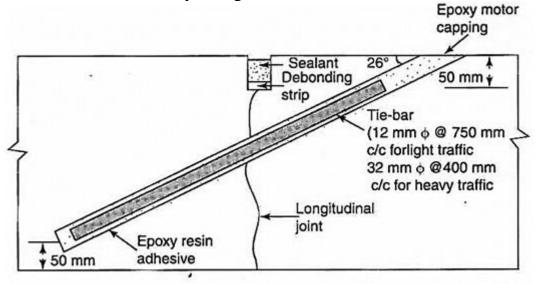
FIG. 10.9 Crack repair by cross-stitching
