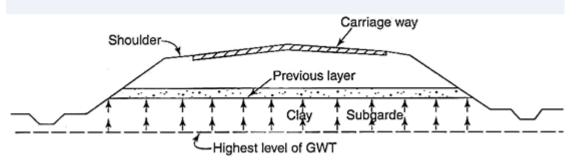
Fig. Capillary cut-off for a clayey subgrade
