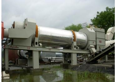
Fig. Mixing Chamber
