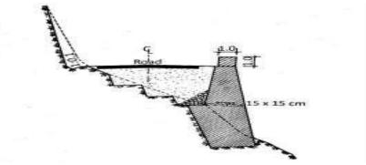
Typical Cross Sections of Embankment with retaining walls
