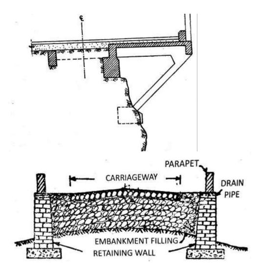
Fig: Fully In Embankment
