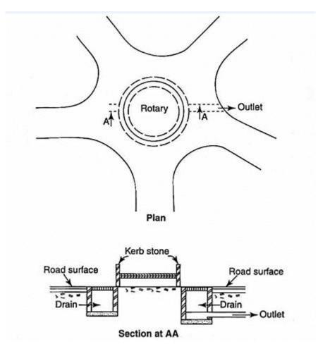
Fig. Typical drainage arrangement at a Rotary
