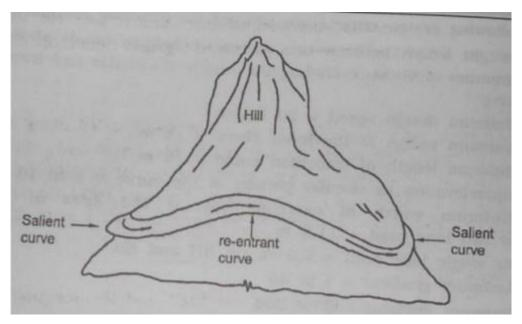
Schematic dig. of Re-entrant curve
