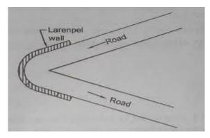
Schematic dig. of Salient curve
