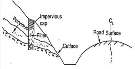
Fig. Subsurface drains at cut slope to control seepage
