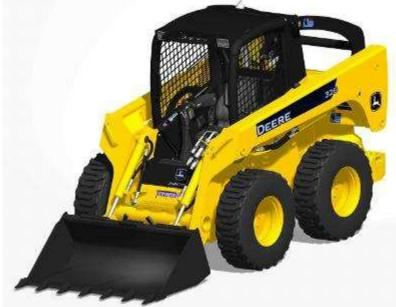
Fig. Skid steer loader
