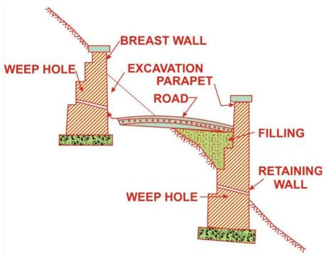
Fig. Retaining wall and breast wall
