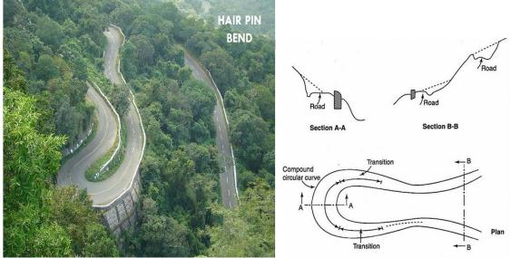
Schematic dig. of hair pin bend curve
